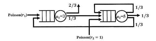
A packet-switched Jackson network routes packets among two routers according to the routing probabilities shown above. Notice that there are two points at which packets enter the network and two points at which they can depart. **A.** What is the maximum allowable rate  $r_1$  that the network can tolerate? [8 marks]
