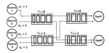
Consider the above system with four flows and four links. The demand for the four flows are 1, 4, 3 and 2 (Mbps) and the capacity of the four links are 2, 4, 5 and 3 (Mbps), respectively.
